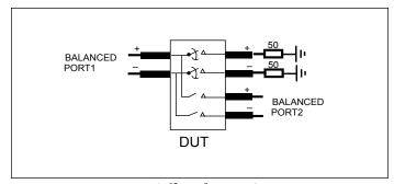
Fig 2. Off-Isolation Setup
