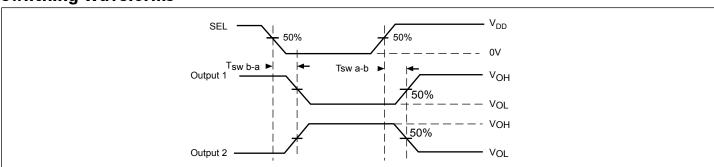
**Voltage Waveforms for Select Timing**
